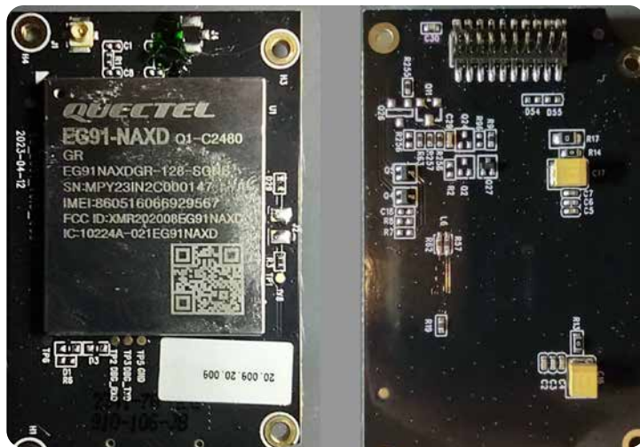
Figure 21: Quoctel EG91-NAXD on Trail Camera's PCB
