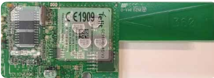
Figure 14: GSM Telit GE910 Cellular Board Transparency Overlay
