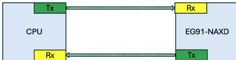
Figure 43: Inter-chip Communications Example
