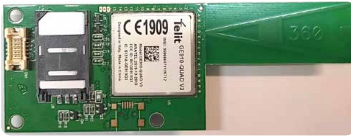
Figure 12: GSM Telit GE910 Cellular Board Obverse Image
