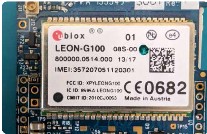
Figure 6. U-Blox LEON-G100 Cellular Module
