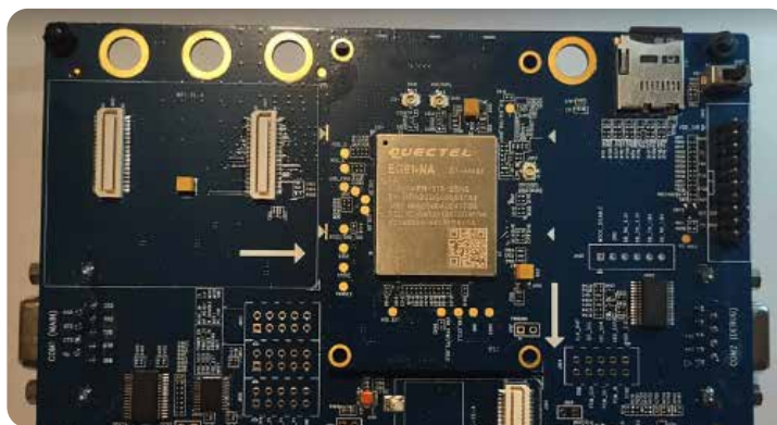
Figure 11. Quectel UMTS&LTE-EVB-KIT with an EG91-NA module
