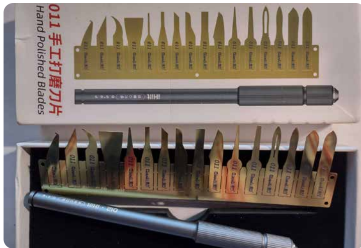
Figure 22: Thin Blades for Removing Components
