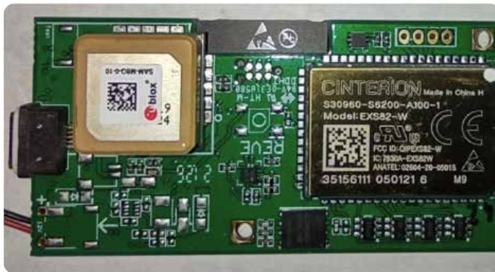
Figure 4. Cinterion Cellular Module in GPS Tracker
