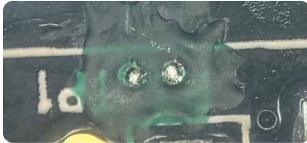
Figure 33: Tinned Repair Trace Pads and Set UV Mask
