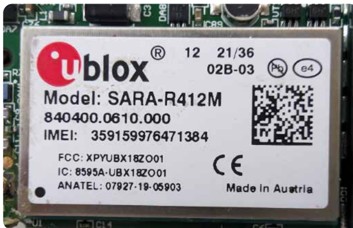
Figure 5. U-Blox SARA-R412M in GPS Tracker
